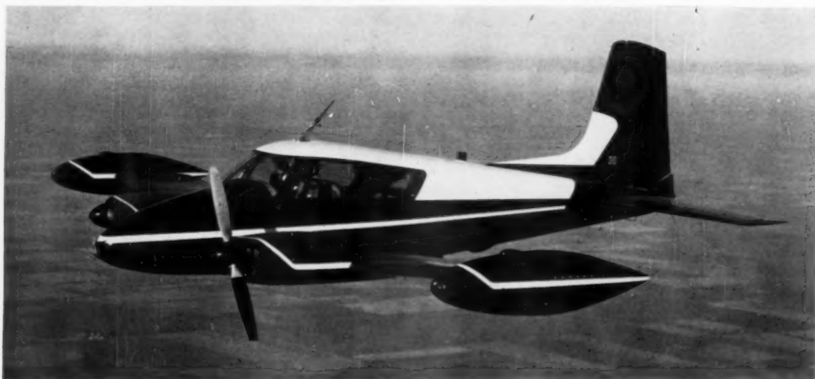
CESSNA 310 handles easily on one engine. Care must be taken to maintain proper trim, but headings can be held within 1-2 deg.
